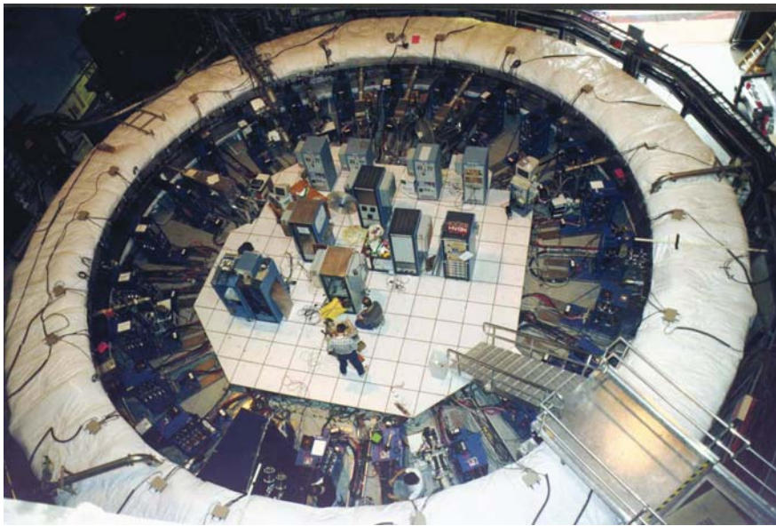
Fig. 6.2. The Brookhaven National Laboratory muon storage ring. The ring has a radius of 7.112 meters, the aperture of the beam pipe is 90 mm, the field is 1.45 Tesla and the momentum of the muon is p_\mu = 3.094 \text{ GeV}/c . Picture taken from the Muon g - 2 Collaboration Web Page http://www.g-2.bnl.gov/ (Courtesy of Brookhaven National Laboratory)
